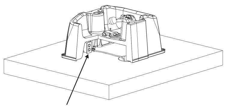
Have a qualified electrician install a properly grounded receptacle outlet, acceptable for outdoor use and protected from the rain and snow.
