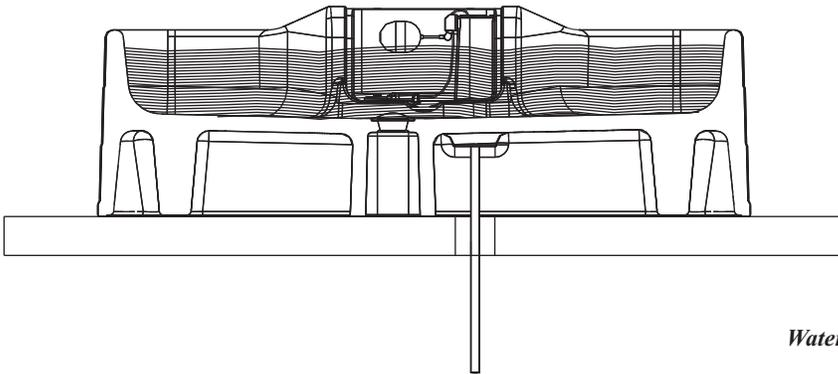
**Water Pressure:** Please note the valve is appropriate for water pressure up to 55 psi.
