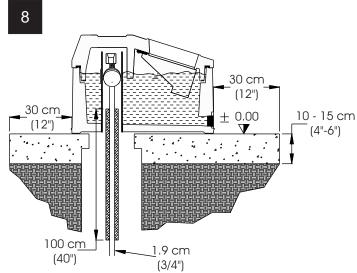
Water Pressure: Please note the valve is appropriate for water pressure up to 55 psi.
