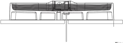
Water Pressure: Please note the valve is appropriate for water pressure up to 55 psi.
