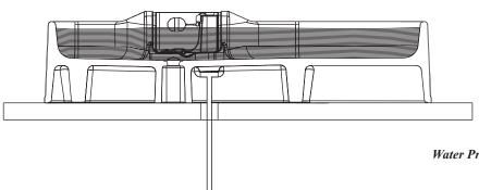
Water Pressure: Please note the valve is appropriate for water pressure up to 55 psi.
