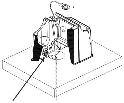
Have a qualified electrician install a properly grounded receptacle outlet, acceptable for outdoor use and protected from the rain and snow
