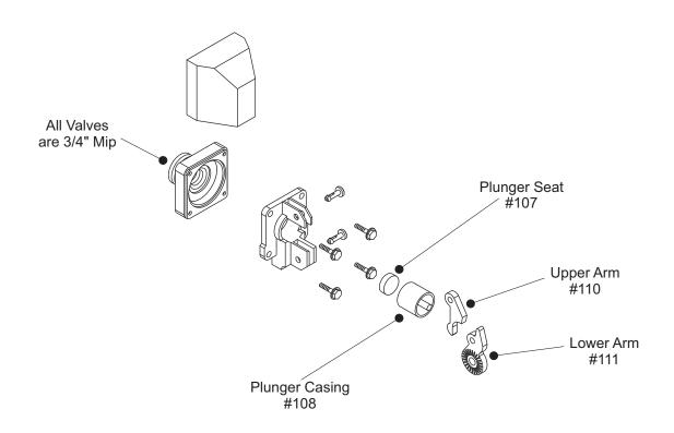
\* Approximate water flow rate of the Float and Valve System with a standard 40-60 psi is 5 - 7 gallons per minute.
