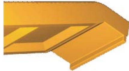
* rendering demonstrating underside of slide face, showing the bolt through attachment areas for DWFS (Double Wall Flat Slide)
