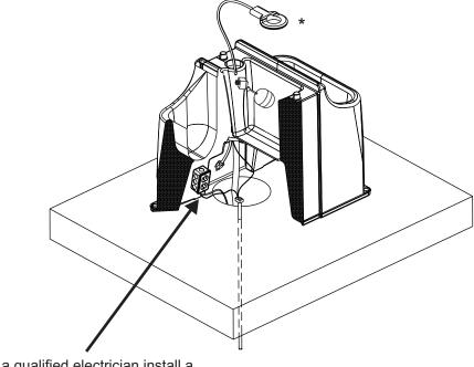
Have a qualified electrician install a properly grounded receptacle outlet, acceptable for outdoor use and protected from the rain and snow
